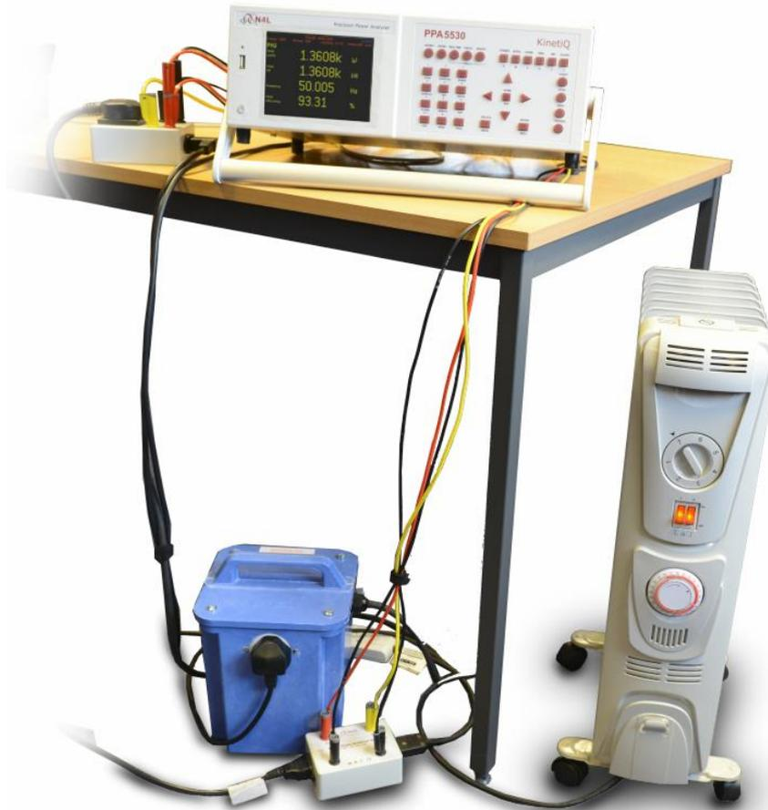
For 3 Phase transformers two N4L PPA5530 can be used in a master slave configuration for 6 phase analysis. This test was performed on a single-phase transformer and the heat was set to maximum.
