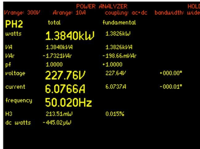
There is a notable difference in the two voltages on the primary and the secondary. We can see a voltage of 232.61V on the primary and 227.76V across the secondary; this is due to the voltage drop across the impedance of the secondary windings of which consists of the resistance of the windings and the leakage reactance of the windings. We have not drawn the vector components of this impedance for simplicity, but it must be taken into account.
