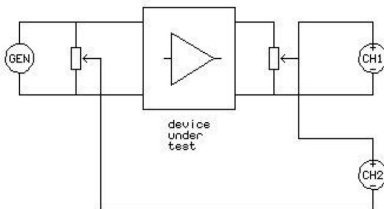
NB. only one attenuator is needed in any given test – use on the input if the forward gain of the DUT is 1 or lower, use on the output if the gain is greater than 1. The attenuator should be of low impedance so that the capacitance of the leads and inputs does not filter the signal.
