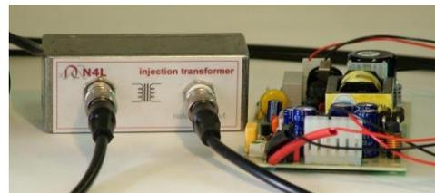
To effectively measure the relative gain and phase of the injected signal, frequency components other than that of the injected frequency must be rejected and this is best achieved using a DFT (Discrete Fourier Transform) on the measured data from CH1 and CH2 as each selected frequency is injected.
