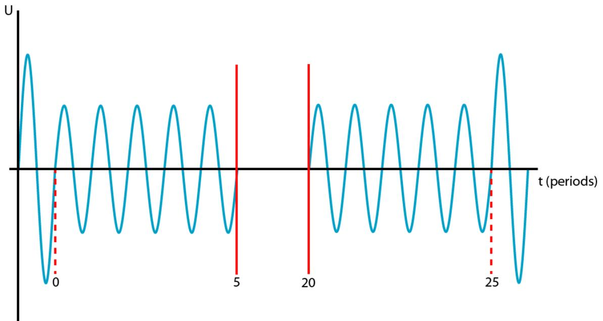
Figure 2 - Voltage Dip example - 70% for 25 cycles
