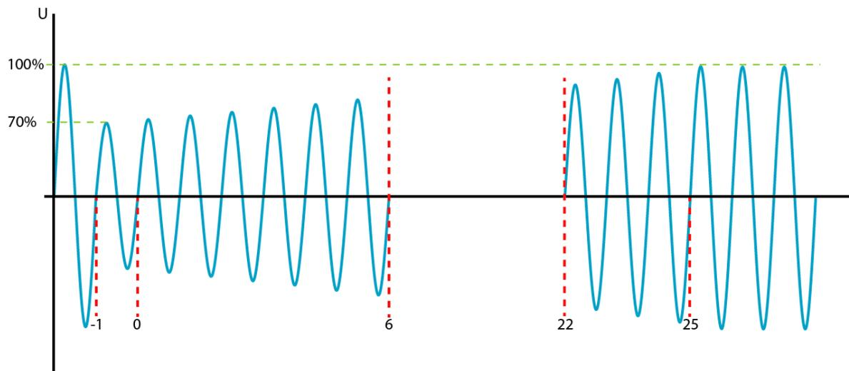
Figure 4 - Example Voltage variation waveform
