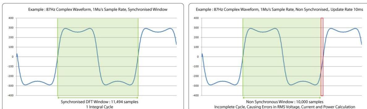
N4L Proprietary Dynamic Synchronous Windowing
