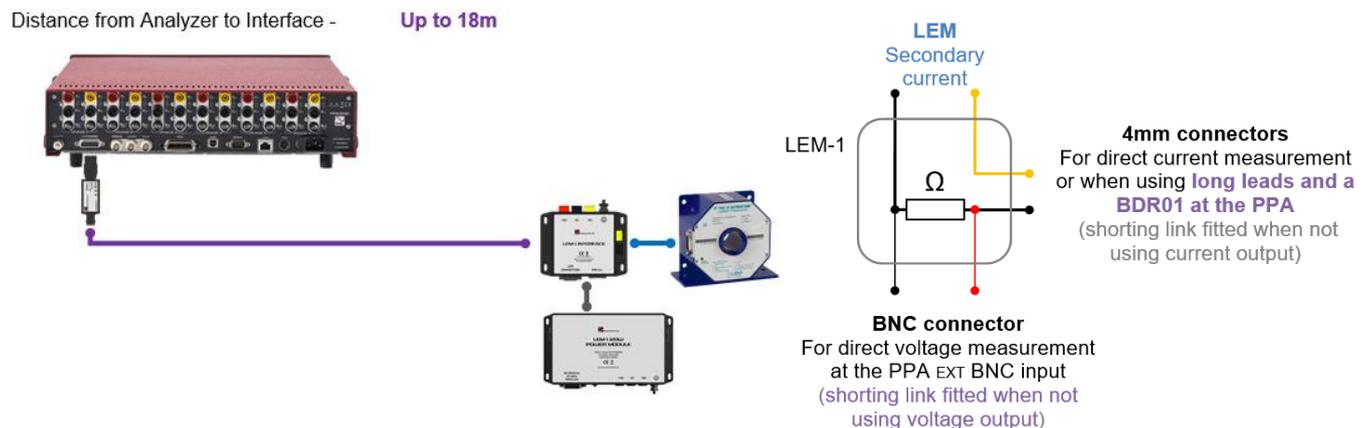
An additional advantage of this connection technique for applications involving a large distance between the measurement instrument current transducer, it that the long cable length uses coaxial wire rather than multicore DSUB to DSUB cable, so there is superior resilience to residual electrical noise while also being more flexible.
