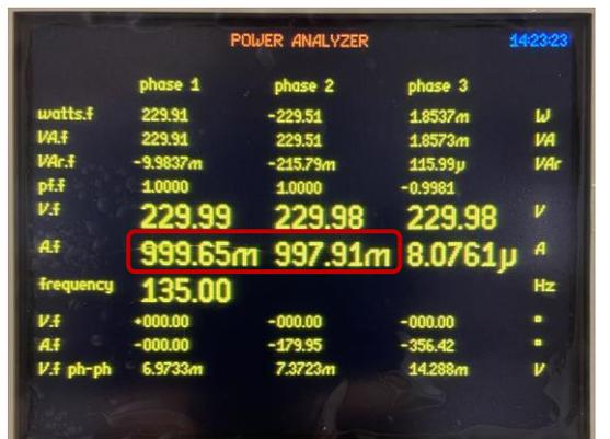
Referencing measurements to the ISO17025 accredited Fluke 6105A, we can produce an accuracy / linearity table.
