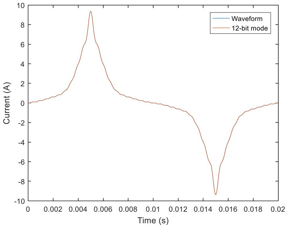
Figure 3: Example IEC waveform with a 50Hz fundamental.
