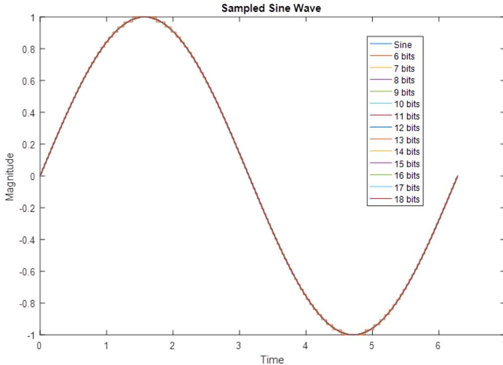
Figure 1: Quantised sine wave from 6 to 18 bit resolution.
