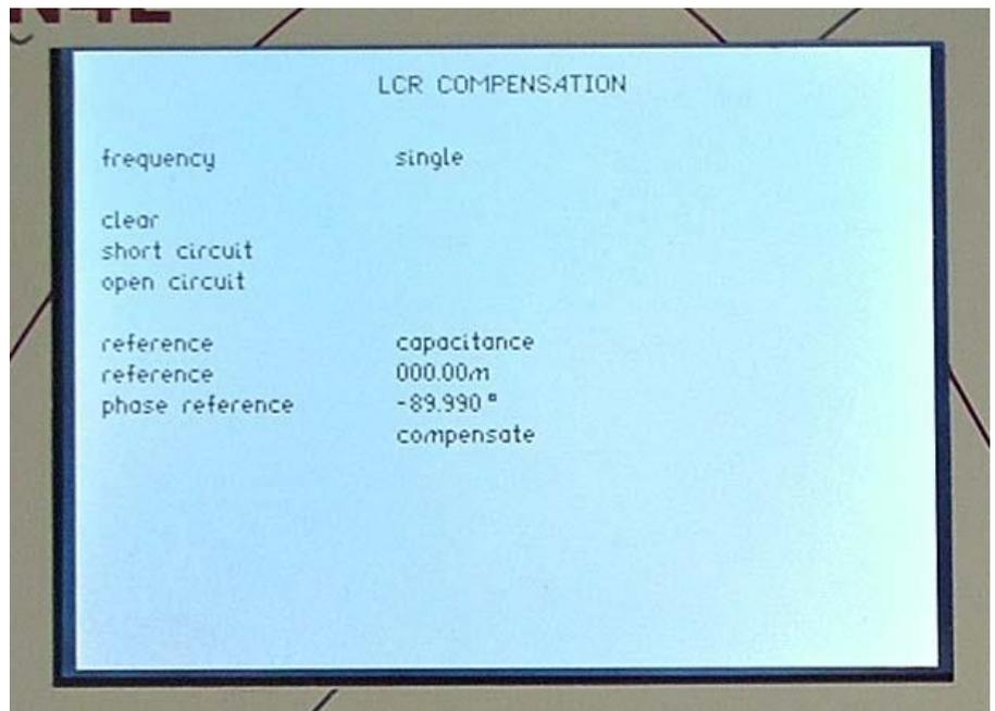
As we presently want to measure capacitance at a relatively low frequency, it should only be necessary to implement 'open circuit' compensation, therefore this is selected using the navigation arrow keys and when a flashing cursor is around the 'open circuit' option, the ENTER button is pressed on the PSM front panel to activate the open circuit compensation process. At this point, the PSM will step through each of the four shunts within the IAI and open circuit compensation will be applied.
