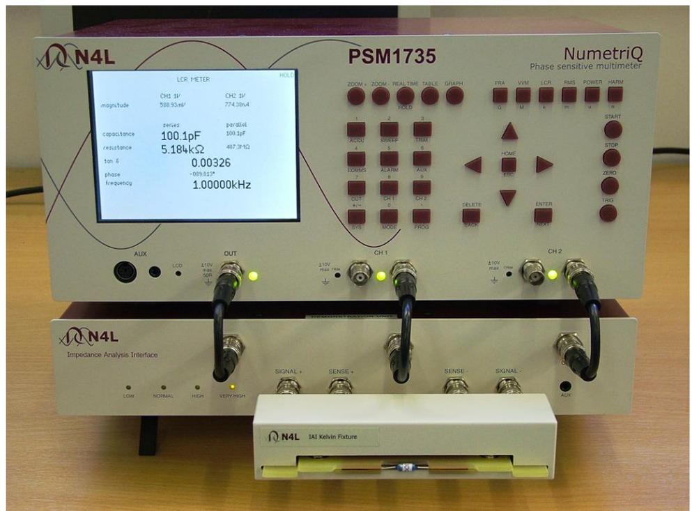
When measuring components that exhibit low impedance, for example inductors at low frequency or capacitors at high frequency, it will also be necessary to apply short circuit compensation.
