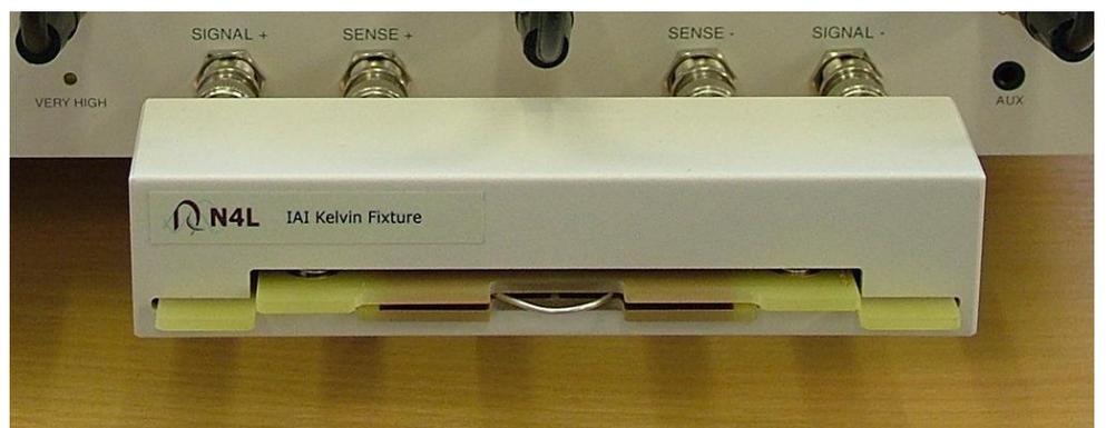
The short circuit compensation using a similar process open circuit described above but this time, a single piece of wire should be fitted to the IAI Kelvin Fixture as shown here to ensure that connection between each power and sense Kelvin pair is good and also that there is a good short circuit between negative and positive Kelvin connections.
