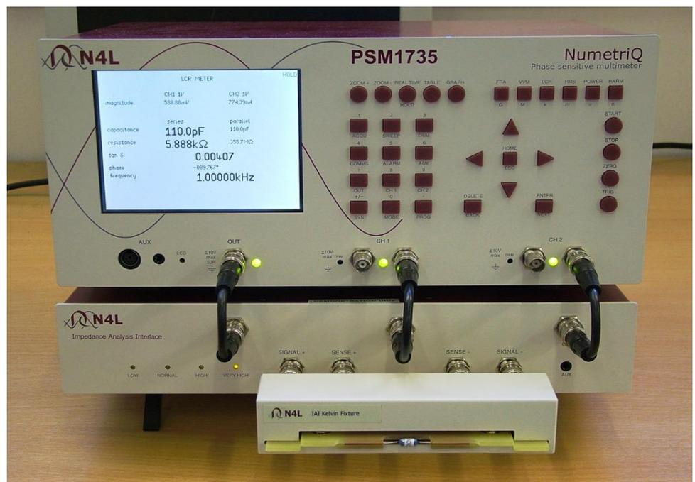
Here, two pieces of single core wire are placed into the Kelvin fixture, one to each side of the fixture so that a good connection between the power and sense Kelvin pairs is achieved.
