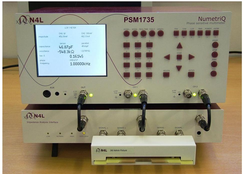
Here, a 100pF capacitor is placed in the IAI Kelvin Fixture. No compensation has been applied.
