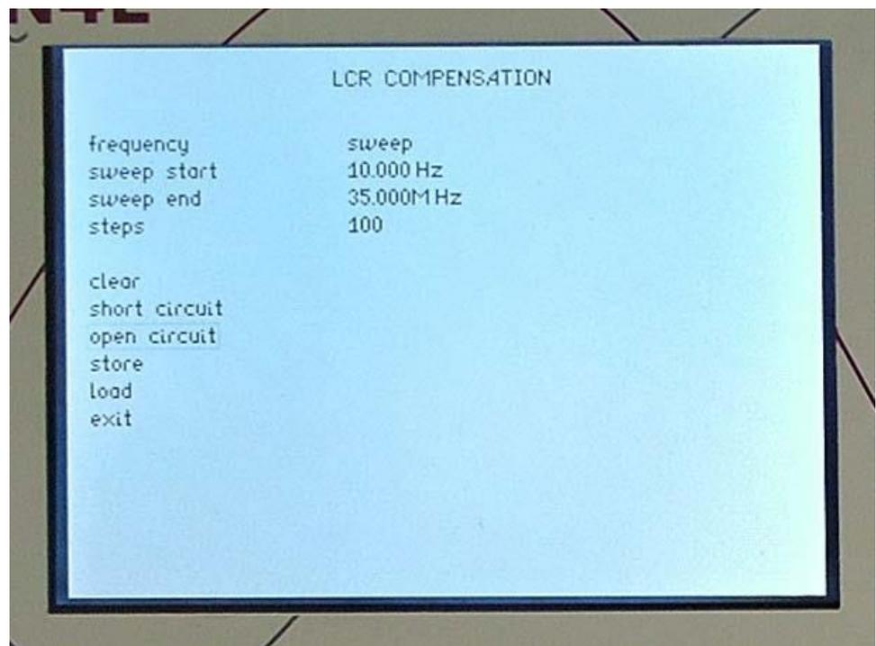
Here it can be seen that 'sweep start', 'sweep end' and 'step' options are presented. As would be expected, sweep compensation covers a frequency range that is at least equal to the range of measurement frequencies that will be required.
