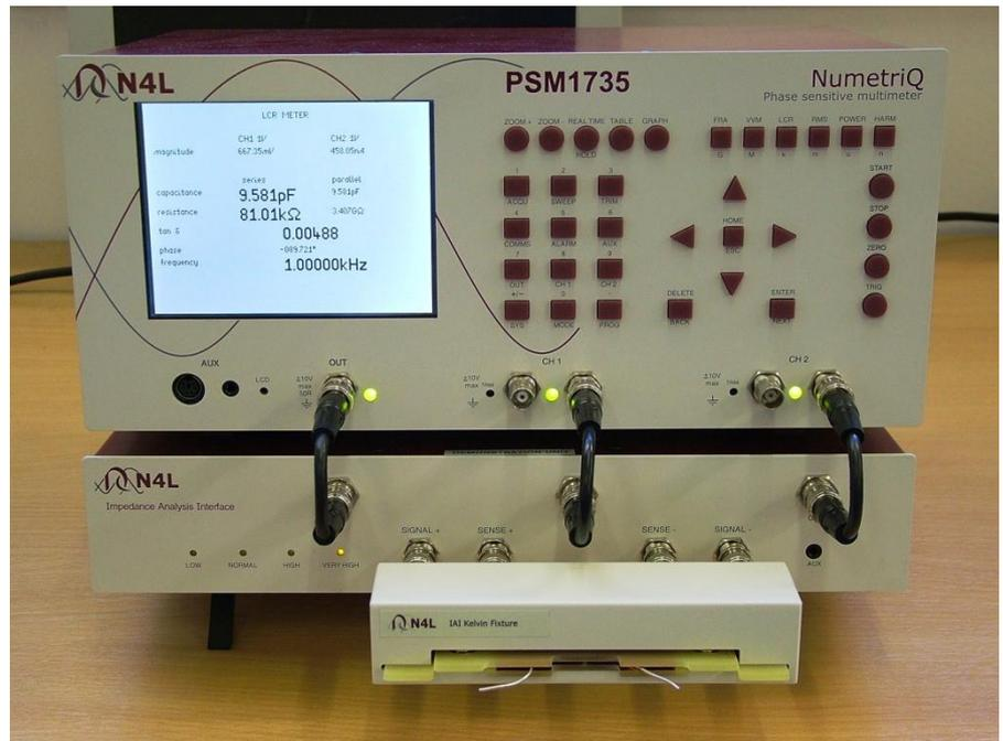
Now, pressing the 'ZERO' button on the PSM will open the Compensation menu as shown here.
