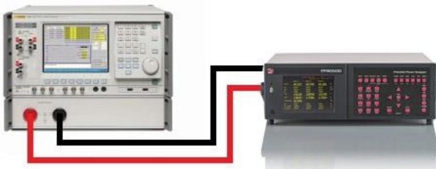
Fig. 4 (Example Calibration setup for the PPA4500 Power Analyzer and Fluke 6105A)
