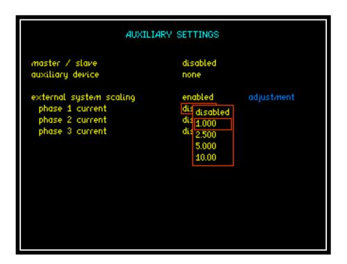
Using the DOWN ARROW selects shunt value, press ENTER and in blue the adjustment is shown Press ENTER.
