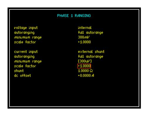
Press DOWN ARROW key and set the shunt value to actual value from calibration certificate.
