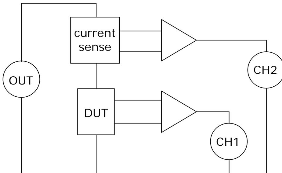
The IAI has 4 selectable 'shunts' to sense the current through the device under test:
