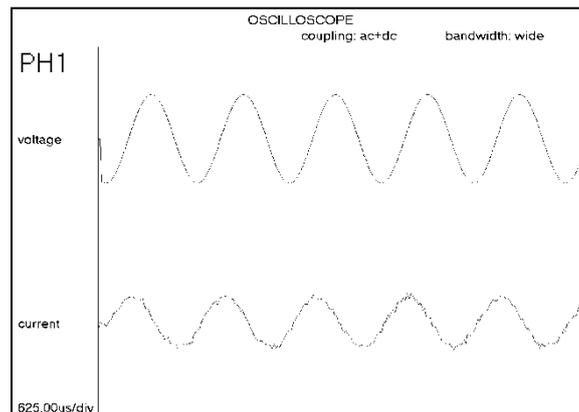
Fig 2 (Correct current waveform)
