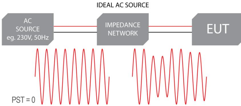
In a perfect or 'ideal' system, the AC source providing power would have no impedance or distortion and therefore flicker measurements would not be influenced by the source.
