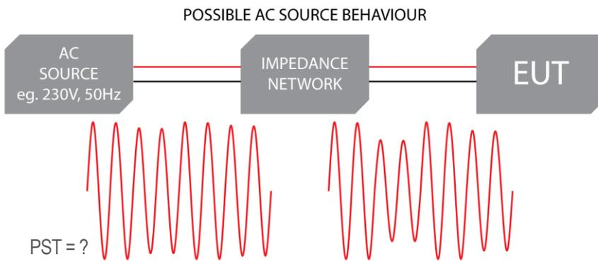
In a real system, the source will have some level of impedance and some level of distortion, so EUT load change will have some influence on the signal applied to the impedance network.
