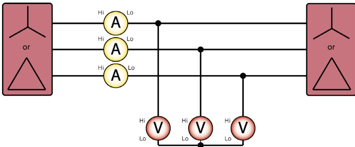
The above picture illustrates the 3 Phase 3 Wattmeter method of power measurement. This is the easiest to understand as the power analyzer will be taking instantaneous, separate measurements of phases 1, 2 and 3. The sum of the three phase powers will equal the total power.
