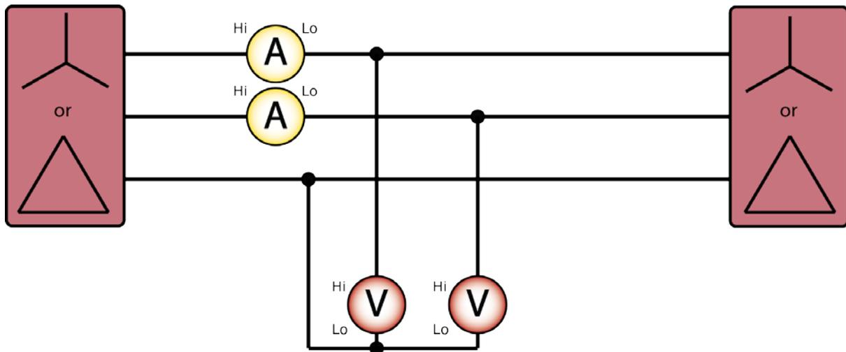
Above is the 3 Phase 2 Watt meter method, this method enables the user to utilise the third phase of a 3 phase power analyzer for a DC bus for example, yet the user is still able to make 3 phase measurements with only the first two channels of the power analyser.
