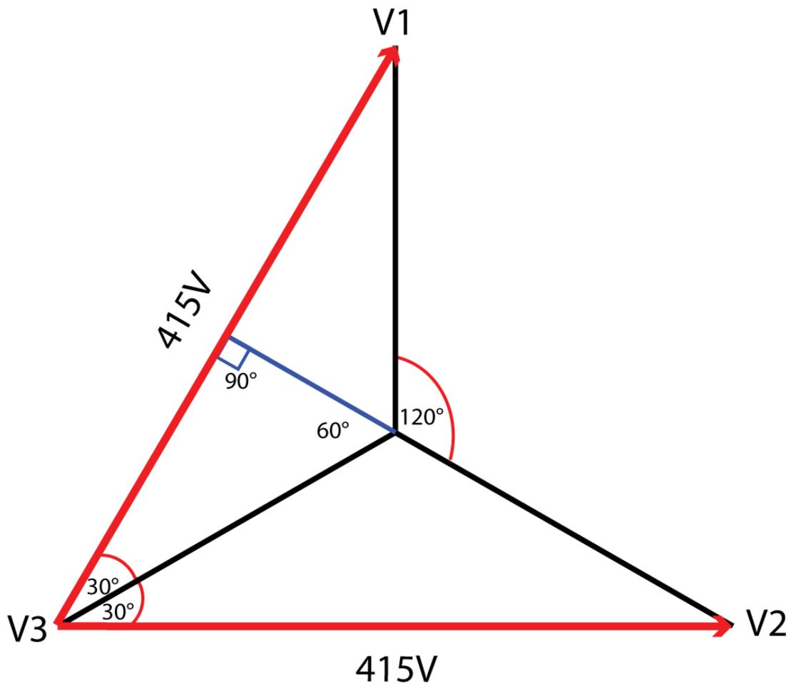
If we now look at the two voltage vectors we are measuring with 3 Phase 2 wattmeter on their own, we can calculate the total voltage by adding the vectors.
