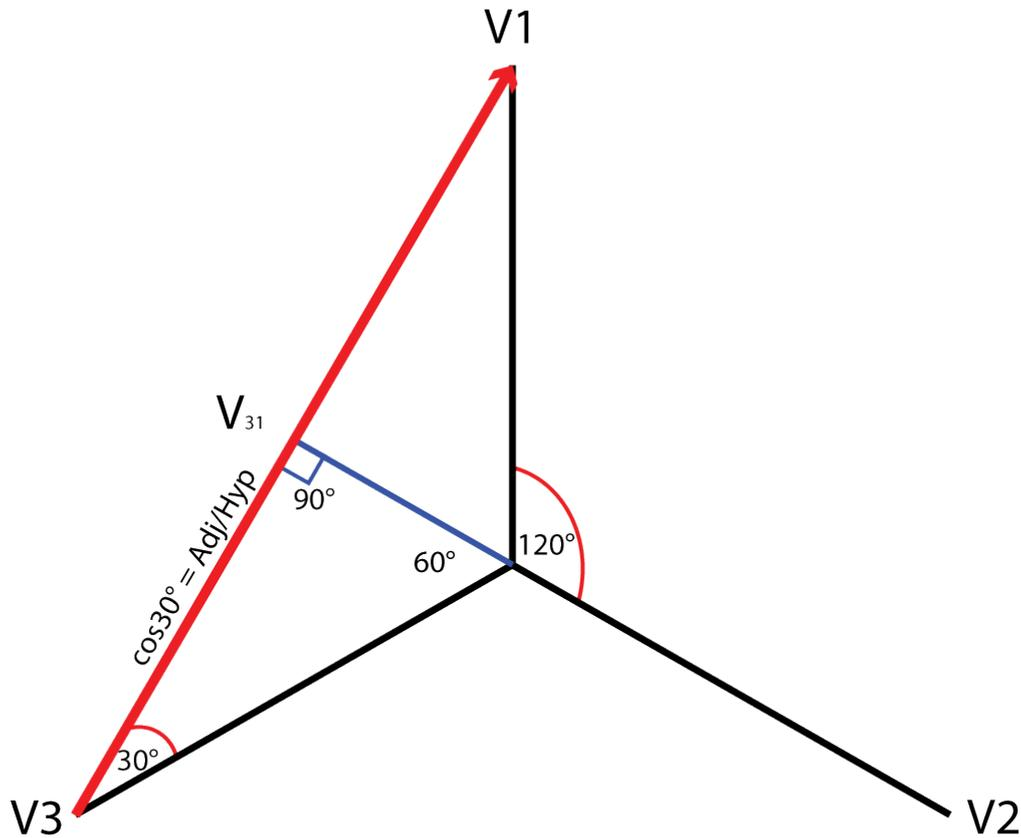
If Voltage was 1V on all phases we can calculate a ratio metric relationship between line to neutral and line to line.
