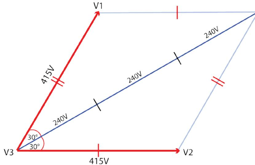
This should give indication that using the 2 wattmeter method would indeed result in the same total voltage being measured vectorially.
