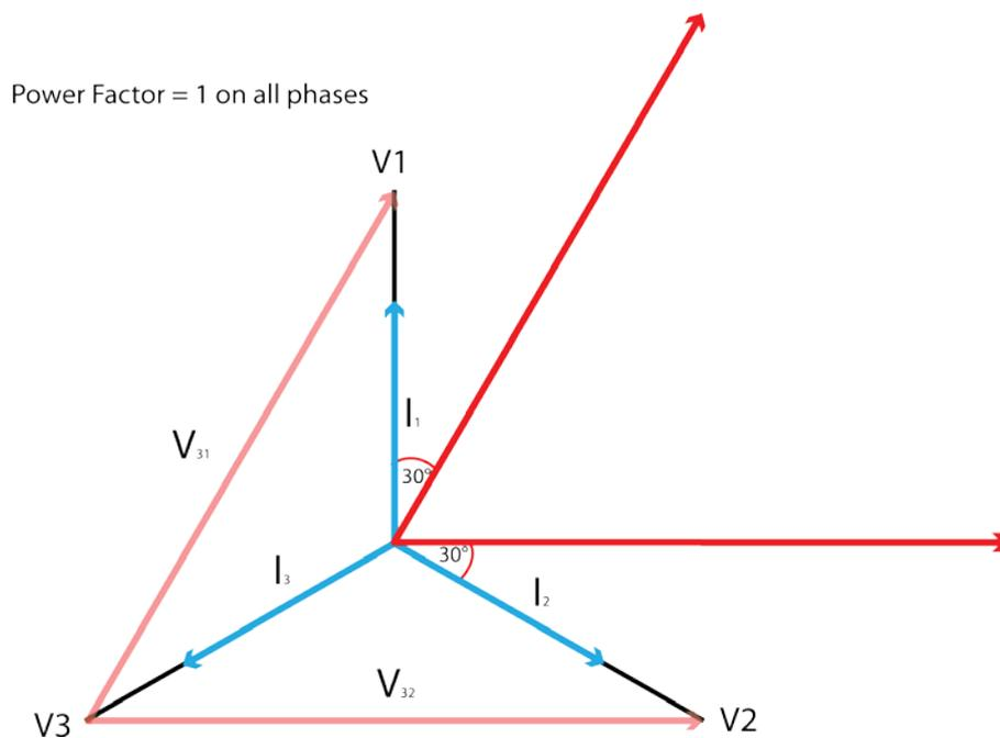
Considering the 30° phase difference between Line to Line voltage and a unity power factor load on every phase, we have to apply this phase difference when computing watts on each wattmeter.
