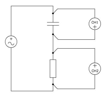
This is the simplest arrangement, using an external resistor as a current shunt.
