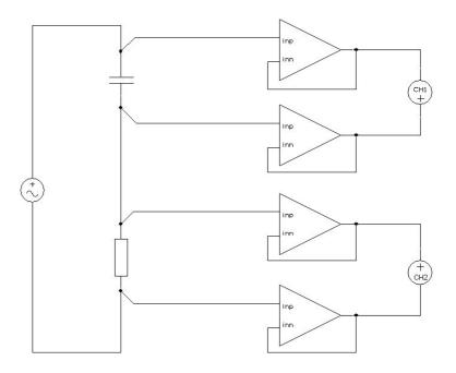
The connections to the instrument are the same as for the passive shunt. The amplifiers must be unity gain stable, and should be selected for high open-loop gain, high frequency performance, and capability of driving capacitive loads if there is significant cabling between the amplifiers and the instrument.
