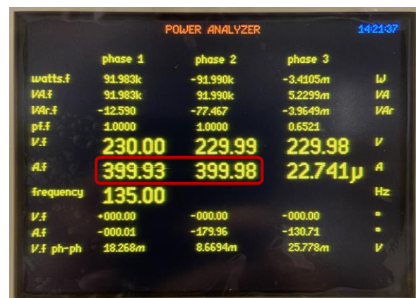
When the corrected scale factor is entered, the WR5000 current measurement correlates with the PPA direct input
