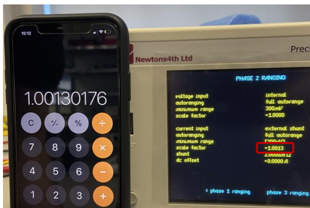
Correction scale factor (1.0013) derived from the measured PH1/PH2 current when using a default 1:1 factor
